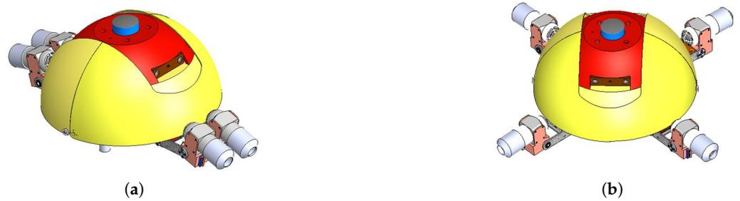
**Figure 3.** Different motion modes of the small spherical robot. (a) “H”-shaped motion mode. (b) “X”-shaped motion mode.
